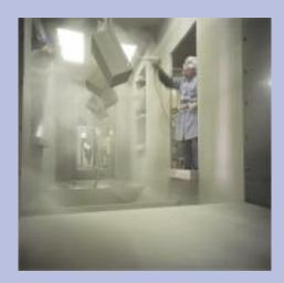
Since 1991, Global has used a powder paint coating process to produce beautiful finishes on chair and panel frames, filing products and storage cabinets. Powder coating provides a high quality finish with excellent chemical and corrosion resistance. It is also environmentally friendly.
